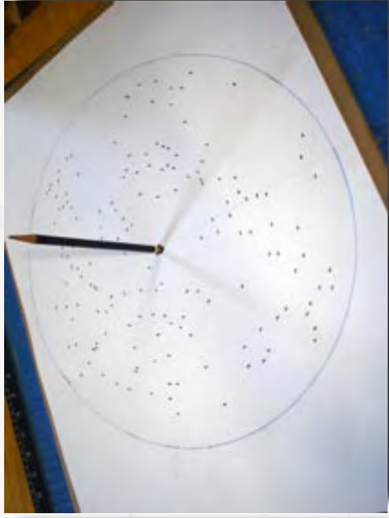
Using this approach and the Tines-Template, the marks are guaranteed to coincide with the Porter Music Box's Tine Positions. In this photograph, we are now looking at the Music! Chills!
