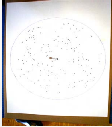
Once the white paper has been inked, the Times-Template is then once again... painstakingly rotated over the dots. This time, the Sharpie is used to fill in the exact rectangular dimensions for the punch on each occurrence.
